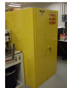
Flammable chemicals storage cabinet
