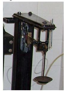
The slide weight may be moved to balance the system to a negative weight (arm in the down position). The valve is then closed on the tank. The arm is watched for movement, and as the arm trips from the low position to the high position, the stopwatch is started. An appropriate mass is added to the weight pan, moving the arm back to the low position. The stop watch is stopped when the arm again moves to the upper position.
