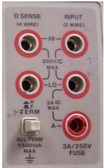
There are 5 connectors used for measurements. The middle connection on the right is the normal common connection for voltage and current readings. The upper connecton on the right is the normal positive connection for ac and dc readings. The lower connection on the right side is for current readings. This is the positive connection for all mA and A readings, with the middle (LO) connection being negative.
