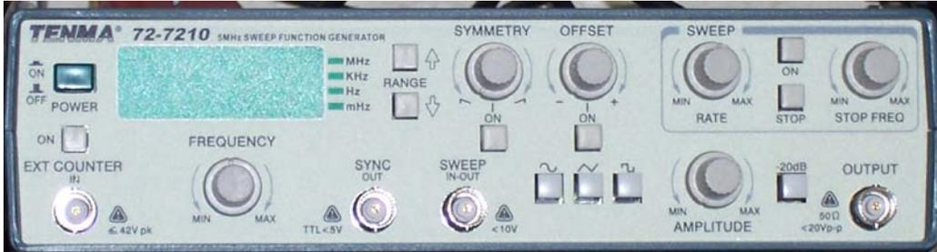
The Tenma 72-7210 Function generator is a single output repetitive function generator. It is capable producing a sine, triangle or square wave with an adjustable frequency and amplitude. The waveform symmetry and base amplitude voltage can be modified, as well as setting the frequency up to sweep between to limits at an adjustable rate.
