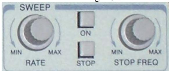
through some range. The SWEEP controls are the portion that controls this. Under normal operation the two buttons are left out, disabling this function. When pressed, the ON button starts the sweep
