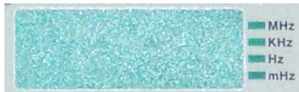
The display indicates the frequency and the lit indicator to the right of the display indicates the frequency range.
