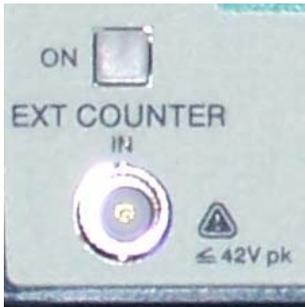
The ON button switches the display to the external counter mode. With the button left out, the display will show the value of the internal frequency generator.
