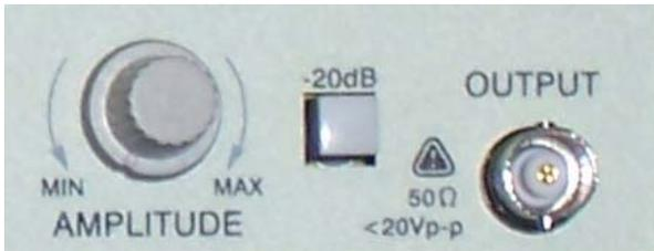
The AMPLITUDE vernier adjusts the peak to peak value of the output signal within the limits. Selecting the -20dB button will lower the output range allowing lower peak to peak values. The OUTPUT connector is the location that the signal is actually generated on.
