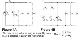
Sensitivity is 400 times greater than an IC thermocouple. Thermistor values as high as 30 mV/°C are common. In addition, output voltage can be applied to a recorder or digital voltmeter to produce a precise, sensitive, direct reading thermometer.
