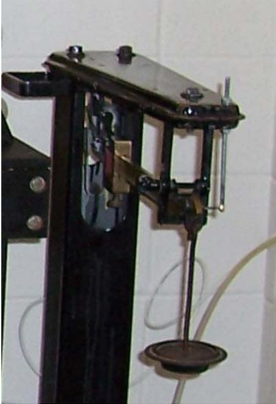
The slide weight may be moved to balance the system to a negative weight (arm in the down position). The valve is then closed on the tank. The arm is watched for movement, and as the arm trips from the low position to the high position, the stopwatch is started. An appropriate mass is added to the weight pan, moving the arm back to the low position. The stop watch is stopped when the arm again moves to the upper position.
