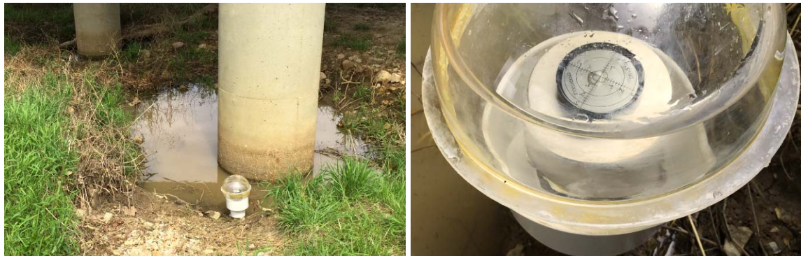
Figure 9 The Prototype APUS Placed next to a Bridge Pier
