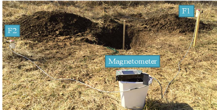
Figure 7 Overall Arrangement of Resetting Tests
