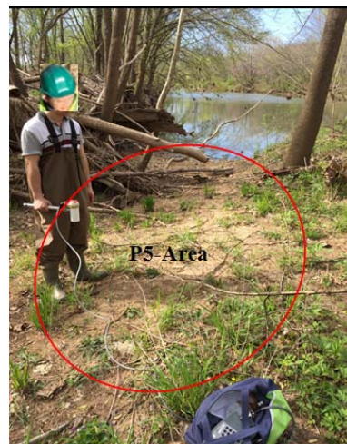
Figure 6 Ambient Magnetic Field Measurement near Pier 5
