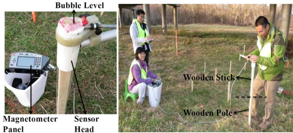
Figure 4.10. Magnetometer setup and operation.
