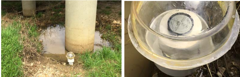
Figure 2.14. The APUS prototype placed next to a bridge pier.
