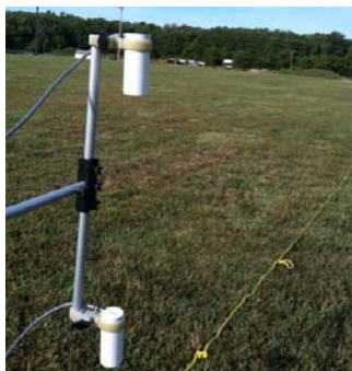
(a) Sensor orientation for vertical gradient measurements
