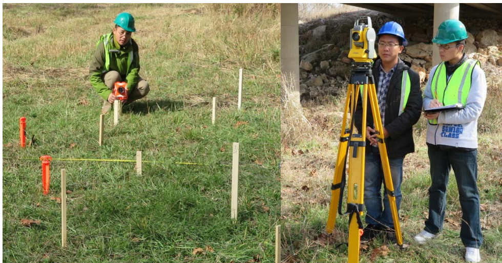
Figure 4 Total Station and Prism for Positioning
