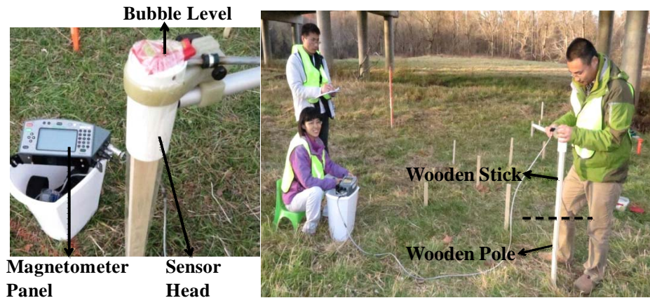
Figure 6 Magnetometer Setup and Operation
