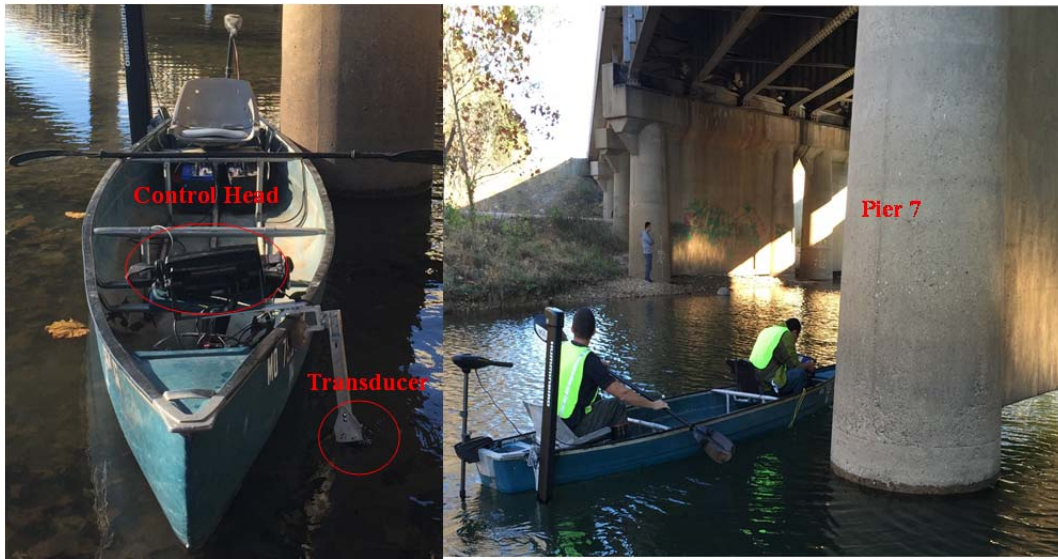
(a) Sonar Instrument Installation
