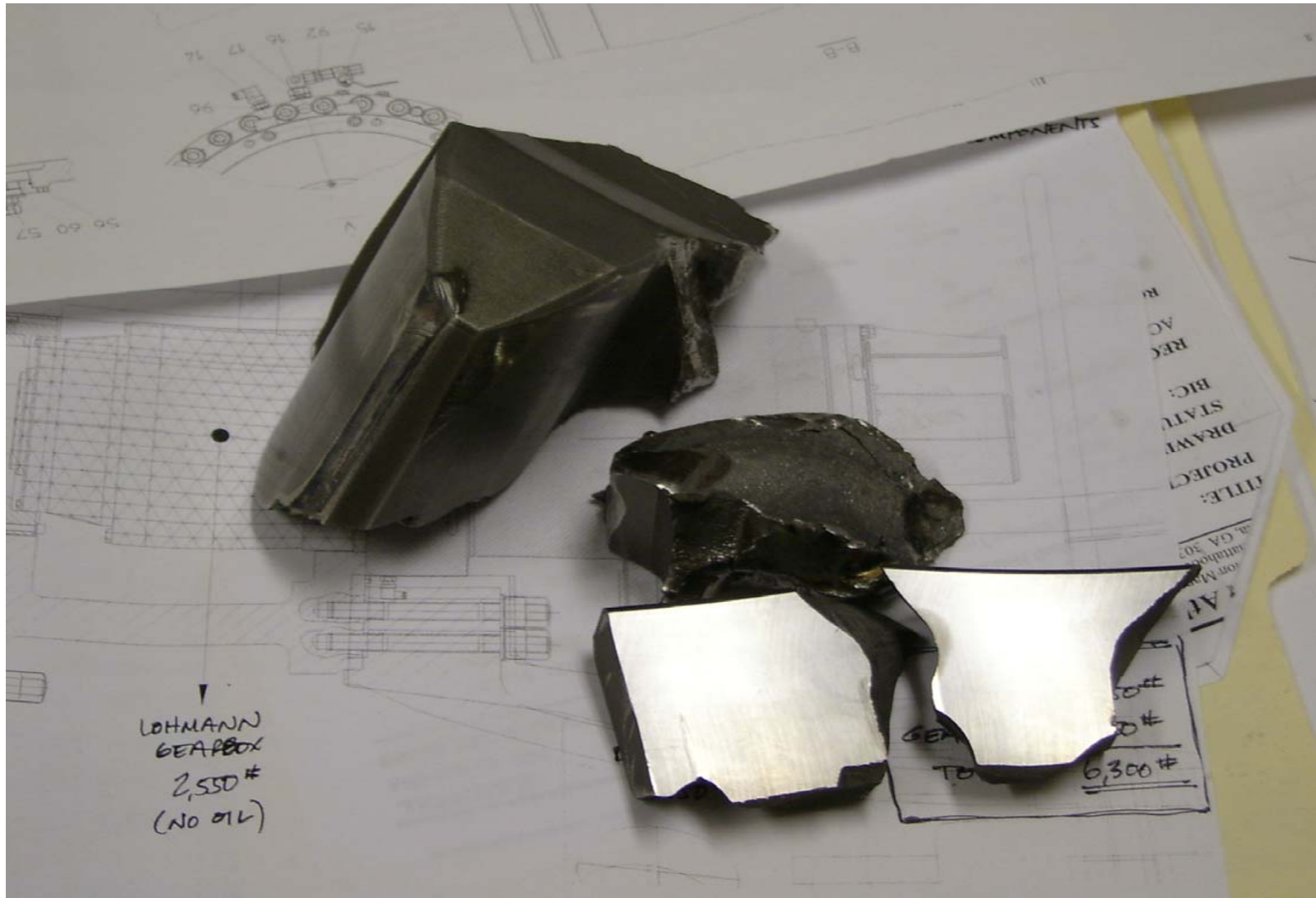
Chunk of gear tooth and broken support bearing outer race
