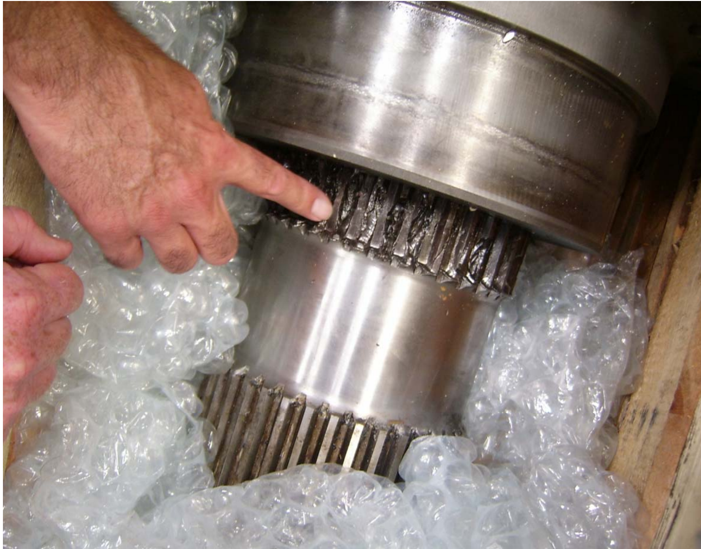
Destroyed when pinion failed
