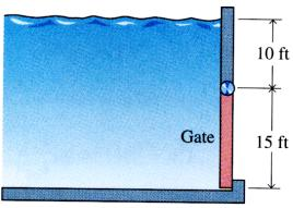
2. The width of the dam shown is 1 ft. Determine the magnitude of the resultant force  $\mathbf{R}$  exerted on the dam by the water. Use  $(=62.4 \text{ lb/ft}^3 \text{ for the specific weight of the water.})$
