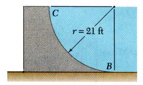
3. For the shaded area shown, determine the radii of gyration  $k_x$  and  $k_y$ .
