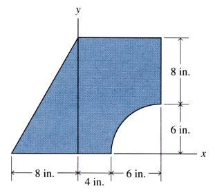
4. Determine the maximum and minimum moments of inertia and the orientation of the principal axes with respect to the axes through the triangle's centroid.
