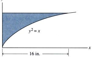
3. Determine the moment of inertia of the shaded area with respect to the x-axis.
