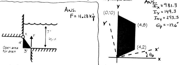
A solid gate with a uniform triangular cross section weighs 2000 lbs. The gate is submerged in a liquid with a weight density of  $\gamma = 112.4 \text{ lb/ft}^3$ . If the hinge at A is smooth, determine the total force (F) required to open the gate when the surface of the liquid is 3 ft above point A. The depth of the gate (into the paper ) is 4 ft.
