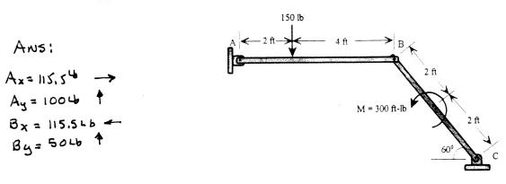
5. Please draw the complete shear and bending moment diagrams for the beam loaded as shown. You must provide numerical values for all pertinent points on the diagrams.
