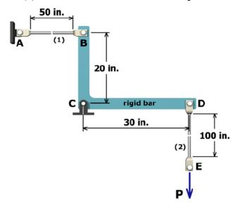
The simple pin-connected structure carries a concentrated load P.
