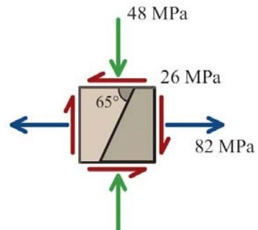
8. Consider a point in a structural member that is subjected to plane stress. Normal and shear stresses acting on horizontal and vertical planes at the point are shown. Determine the principal stresses acting at the point. Show these stresses on an appropriate sketch. (12 points)
