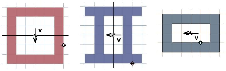
7. (7 points) Determine the following values used for finding the maximum horizontal shear stress  $\tau = VQ/Ib$ .
