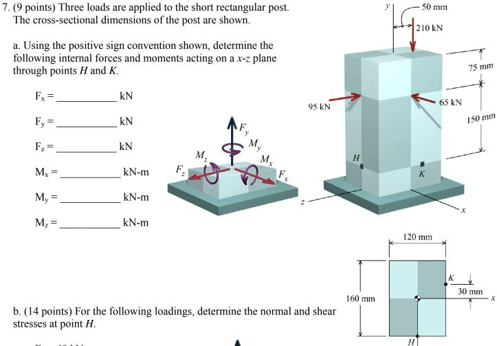
$F_x = 48 \text{ kN}$   $F_y = 0 \text{ kN}$   $F_z = 73 \text{ kN}$   $M_x = 3 \text{ kN-m}$   $M_y = 0 \text{ kN-m}$  $M_z = -2.5 \text{ kN-m}$
