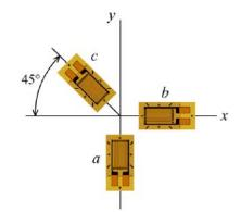
3. (8 points) The strain components  $\varepsilon_x = 390\mu$ ,  $\varepsilon_y = 820\mu$ , and  $\gamma_{xy} = -560\mu$  are given for a point on the free surface of a machine component. The modulus of elasticity for the material is E = 73 GPa and the Poisson's ratio is  $\nu = 0.30$ . Determine the stresses  $\sigma_x$  and  $\tau_{xy}$  at the point.
