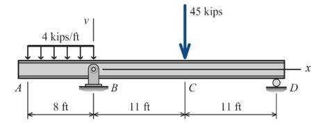
18. The beam shown consists of a *W* 610×140 structural steel wide flange shape [E = 200 GPa;  $I = 1,120 \times 10^6$  mm<sup>4</sup>]. Determine the magnitude of the reaction at *B* if w = 75 kN/m and P = 160 kN.
