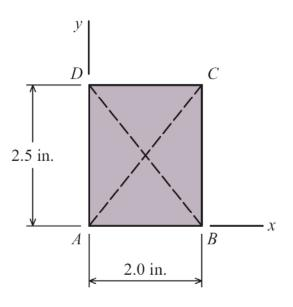
The strain components  $\varepsilon_x = -235\mu$ ,  $\varepsilon_y = -835\mu$ , and  $\gamma_{xy} = 200\mu$ rad are given for a point in a body subjected to plane strain.
