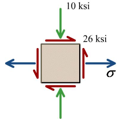
20. Determine the maximum in-plane shear stress and the average normal stress values acting at the point in the previous problem.
