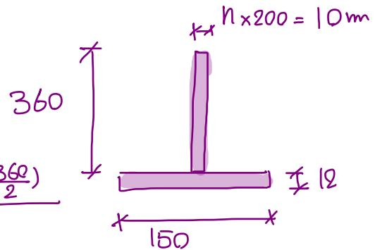
14. The internal shear force  $V$  at a certain section of a steel beam is 80 kN, and the moment of inertia is 64,900,000 mm<sup>4</sup>. Determine the horizontal shear stress at point  $H$ , which is located  $L = 20$  mm below the centroid.
