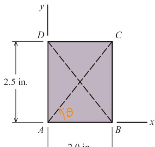
The strain components  $\varepsilon_x = -235 \mu\epsilon$ ,  $\varepsilon_y = -835 \mu\epsilon$ , and  $\gamma_{xy} = 200 \mu\text{rad}$  are given for a point in a body subjected to plane strain.
