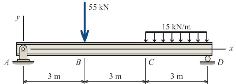
7. Use the graphical method to construct the shear-force diagram and identify the magnitude of the largest shear force (consider both positive and negative). The ground reactions are shown.
