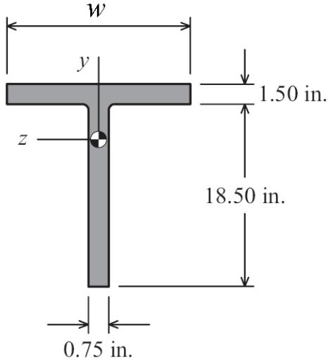
12. If  $w = 5$  in., find the moment of inertia about the  $z$  axis. The centroid of the section is located 2.583 in. from the bottom of the beam.
