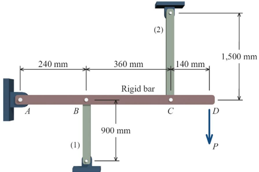
3. Two solid cylindrical rods support a load of  $P = 25 \text{ kN}$  as shown. Determine the normal force in rod (2).
