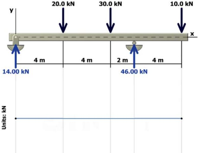
8. Use the graphical method to construct the shear-force diagram and identify the magnitude of the largest shear force (consider both positive and negative). The ground reactions are shown.
