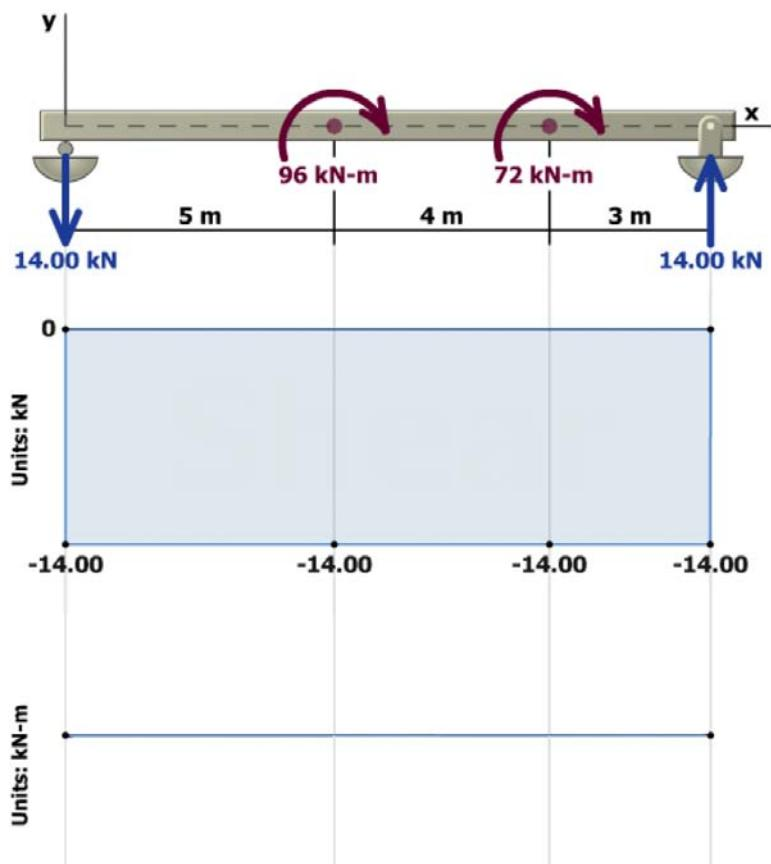
10. Use the graphical method to construct the bending-moment diagram and identify the magnitude of the largest moment (consider both positive and negative). The ground reactions and shear-force diagram are shown.
