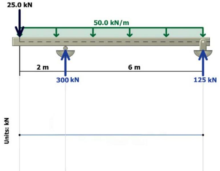
9. Use the graphical method to construct the bending-moment diagram and identify the magnitude of the largest moment (consider both positive and negative). The ground reactions and shear-force diagram are shown.
