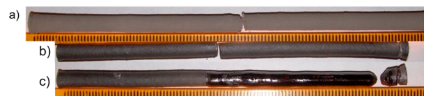
Figure 2. Seed (left) and feed (right) rods used in the crystal growth of \text{Mn}_3\text{Ta}_2\text{O}_8 : (a) presintering; (b) postsintering; (c) postgrowth. Scale marks are millimeters. Approximately 2/3 of the growth ( \approx 3 \text{ cm} ) in part c is a single crystal. The remainder transitions from highly polycrystalline to single crystal along the direction of the growth.
