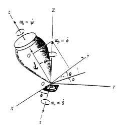
The heavy spinning top shown is a body with an axis of symmetry which is mounted on a ball–and–socket joint at O. Its moment of inertia about its axis of symmetry z is  $I_z$ , its moment of inertia about any axis through O perpendicular to the z-axis is  $I_x$ , the distance from O to the center of mass G is d.
