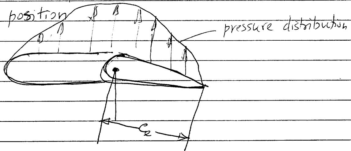
$$H_e = C_{H_e} \rightarrow 8V_c S_e C_e \equiv \text{Hinge Moment}$$
