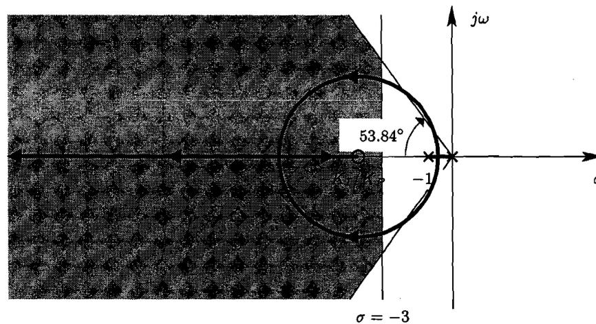
Since a lot of choices for the zero would work, one possible choice is  $K_I/K_P = 4$ . For that choice, the radius is  $r = \sqrt{(-4 - 0)(-4 - (-1))} = \sqrt{12}$ , and the intersection of the root-locus branch and the  $\{\sigma = -3\}$  line is at  $s = -3 \pm j\sqrt{11}$ . The gain at  $s = -3 \pm j\sqrt{11}$  can be determined from the magnitude condition, such that
