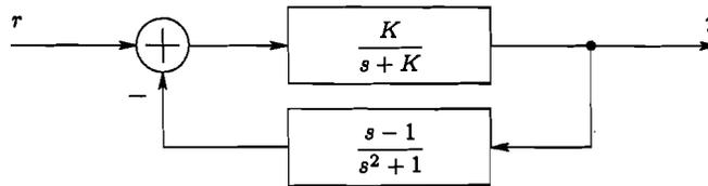
**Solution:** The sketch of the location of the closed-loop poles is the root-locus diagram. However, in this case the open-loop gain of the system is
