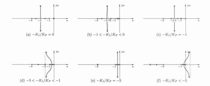
In case (a), the system is no longer type-1. In case (b), the dominant closed-loop real pole is greater than -1. In the cases (d)–(f), the dominant poles all have real parts greater than -2. So the only good option is to cancel the pole at -1 as in the case (c). In other words,
