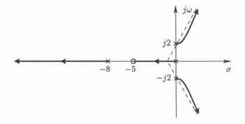
As we observe from the root-locus diagram, there is no value of K that would result in a stable closed-loop system; mainly because the asymptote angles are  $\theta_a = \pm 60^\circ$ , 180°, and there are poles on the imaginary axis.
