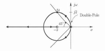
We observe that the radial line and the root-locus diagram intersect. The intersection point,  $s_d = -2 + j2$ , satisfies the damping-constant requirement, and it is also on the root-locus diagram. As a result, we can determine the constant K from the magnitude condition.
