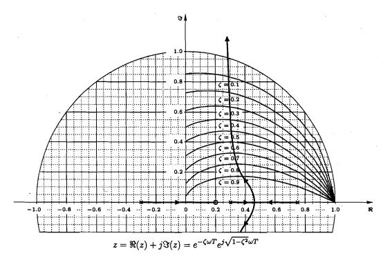
(a) Design the simplest controller, such that the dominant closed-loop poles have  $\zeta = 0.4$ . (15pts)
