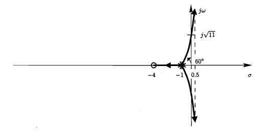
4. Sketch the location of the closed-loop poles for the following feedback control system under a proportionalintegral controller
