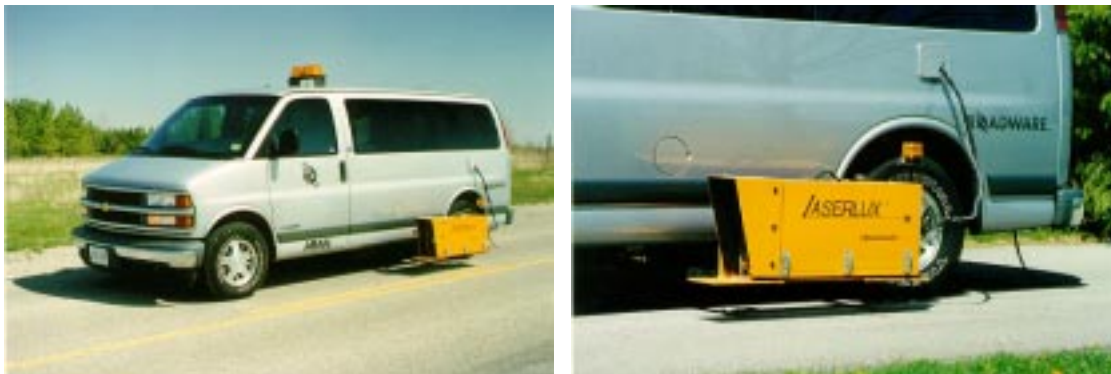
Figure 2. Picture of a Laserlux unit mounted on the side of a Roadware data acquisition platform.
