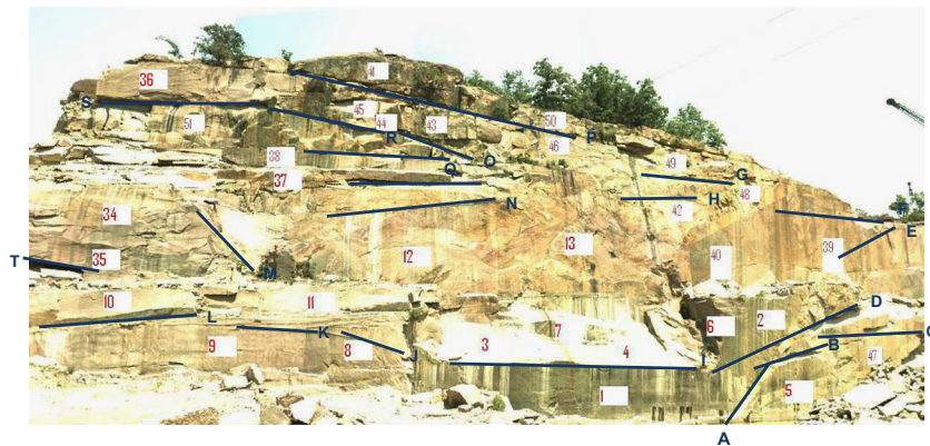
Fig. 4. LiDAR scan of a section of the Red Granite quarry face, showing facets labeled with digits in red ink and white background, and traces labeled with alphabets in blue ink. (For interpretation of the references to color in this figure legend, the reader is referred to the web version of this article.)
