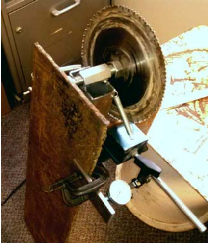
Figure 16. Fixture to move a hinged flat steel plate in increments of 0.001" by rotation a threaded rod, verified by a dial gauge. Note that the plate is hinged at the bottom and tilts forward at the top.
