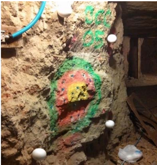
Figure 14: Deformation simulation test. Paint applied to a drift wall in the MST experimental mine.
