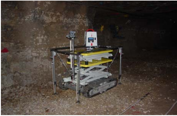
Figure 6: Robotic crawler with remote controlled LIDAR, camera, navigation, lift table, and stabilizing legs, inside the Missouri S&T experimental mine
