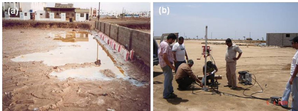
Fig. 11 a Sabkha soil in Jizan and b the dynamic cone penetration used in the sabkha soil in Jizan city
