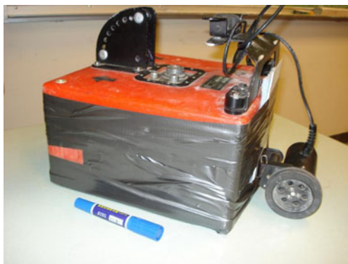
Fig. 4 A wheel was attached to the used 400-MHz GPR monostatic antenna to acquire the data in distance mode while towing the antenna on rock-cut faces
