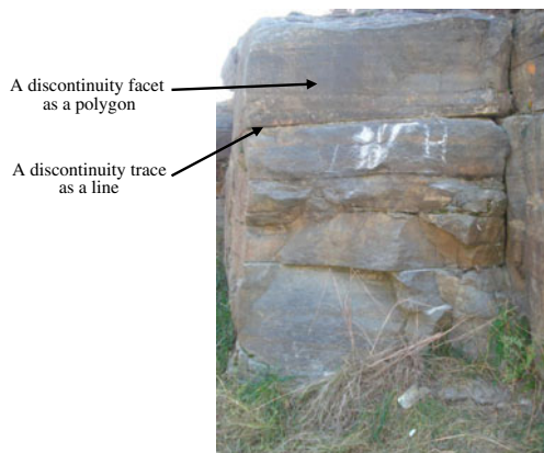
Fig. 1 A rock cut showing both discontinuity traces as lines and discontinuity facets as polygons
