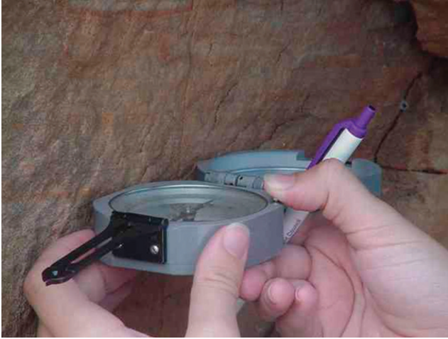
Figure 1. Manual measurements of joints are slow, tedious, expose the user to danger, and are often limited to locations that are easily accessible.
