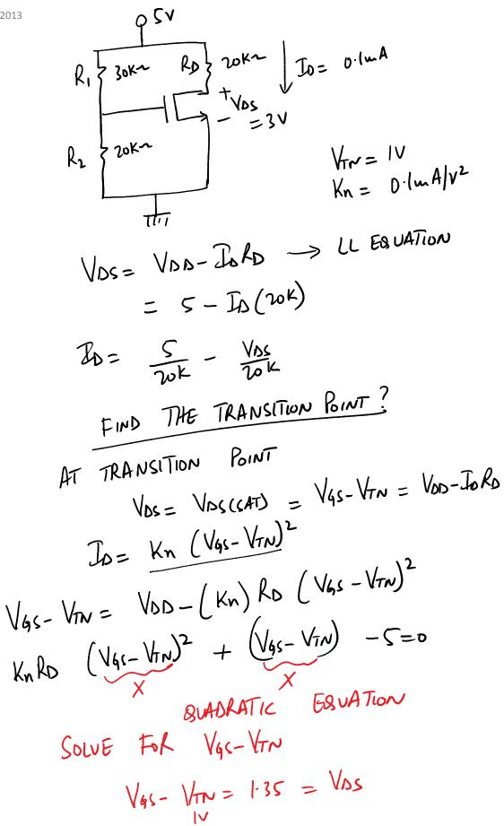
$V_{4s} = 2.35 V$   $J_{0} = (0.1m) (2.35-1)^{2} = 0.182mA$ For  $V_{4s} < 2.35V$  TR IS IN SAT.  $V_{4s} > 2.35V$  TR IS IN TRIODE REGION As  $V_{4s} \uparrow J_{0} \uparrow V_{0s} \downarrow$
