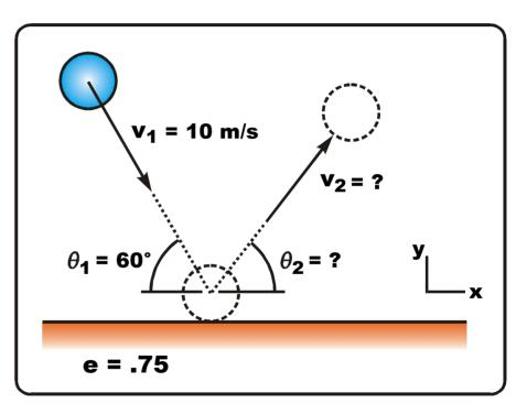
Key step: Resolve the  $v_1$  components.... Resolve the  $v_1$  vector into x and y components:
