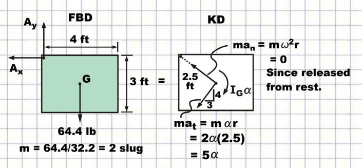
Calculate  $I_G$  for the plate:  $[I_G = (1/12)m(a^2 + b^2)]$
