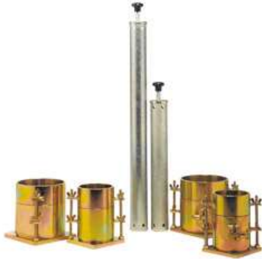
The Modified Proctor Test uses a 10-lb hammer in an 18-inch drop sleeve. Both the original and Modified Proctor test components are shown here
