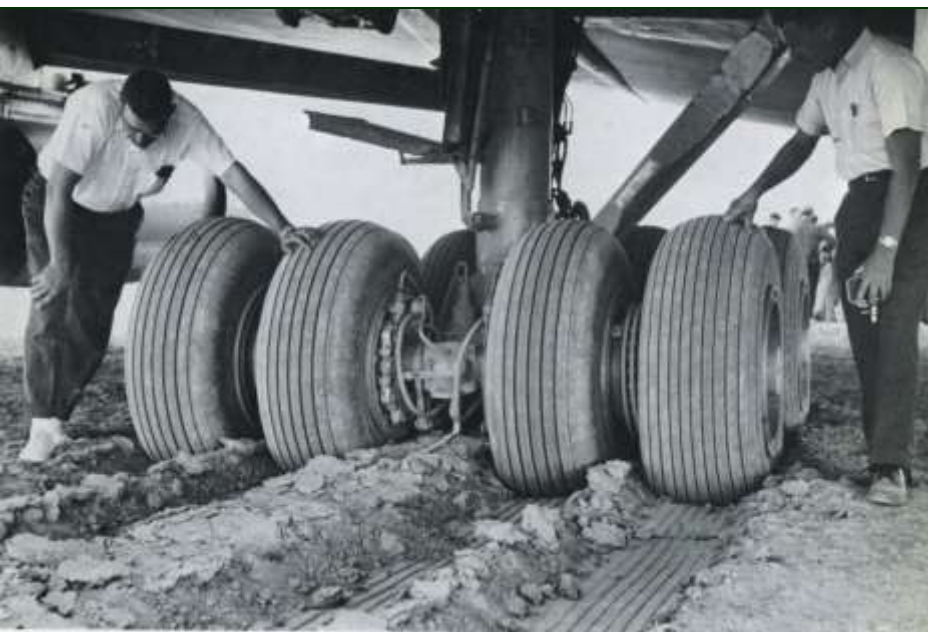
Boeing 707-80 high flotation tire tests at Harper Dry Lake in the Mojave Desert in 1964. It was chosen because it is a “wet” dry lake, with a thin crust about an inch thick, above a soft silt bed. The aircraft’s tires sank about 6 inches (shown below).
