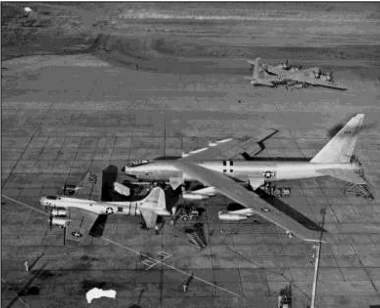
The YB-52 was a giant leap in scale over the heaviest World War II bombers shown here next to it, a B-17 and B-50 (background).
