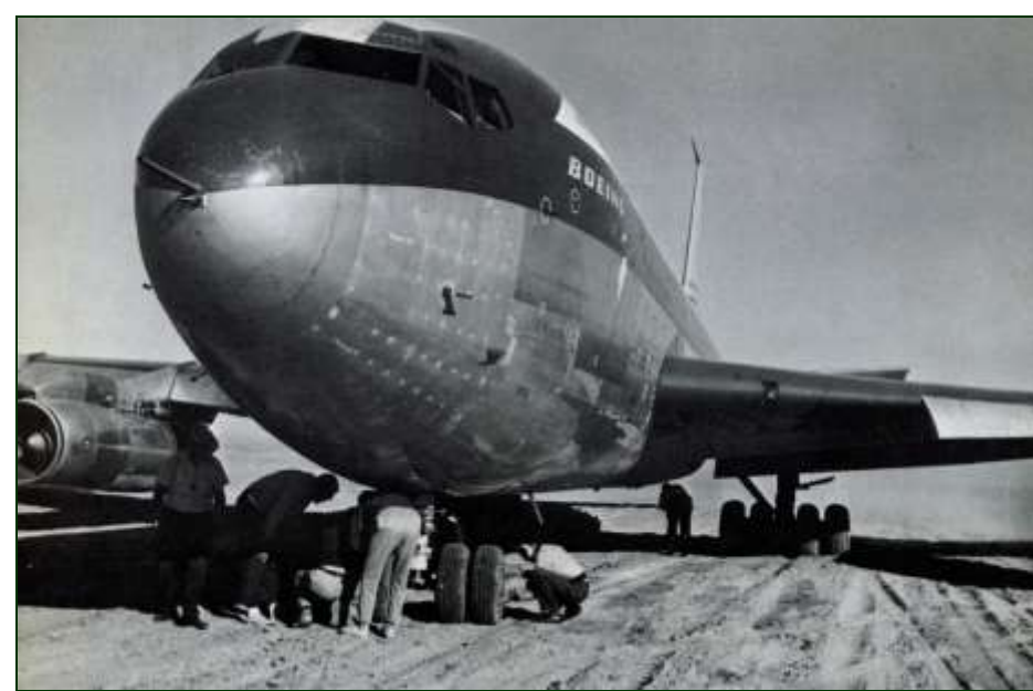
Boeing 707-80 high flotation tire tests at Harper Dry Lake in the Mojave Desert in 1964. It was chosen because it is a “wet” dry lake, with a thin crust about an inch thick, above a soft silt bed. The aircraft’s tires sank about 6 inches (shown below).
