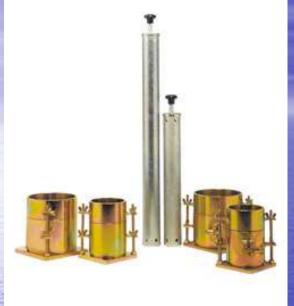
The Modifed Proctor Test uses a 10-lb hammer in an 18-inch drop sleeve. Both the original and Modified Proctor test components are shown here
