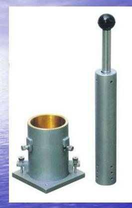
Standard Proctor Compaction
