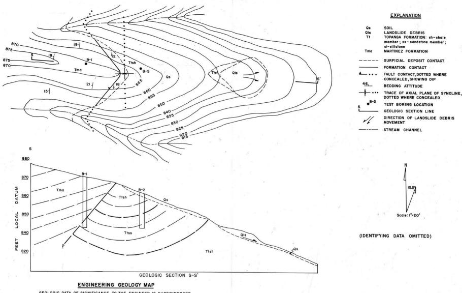
GEOLOGIC DATA OF SIGNIFICANCE TO THE ENGINEER IS SUPERIMPOSED ON THE TOPOGRAPHIC MAP. A GEOLOGIC SECTION IS ADDED TO FACILITATE ANALYSIS IN THREE DIMENSIONS. EXPLANATION OF SYMBOLS SHOULD ACCOMPANY THE MAP. DETAILED DESCRIPTIONS OF THE EARTH MATERIALS ARE USUALLY GIVEN IN THE TEXT OF THE REPORT.
