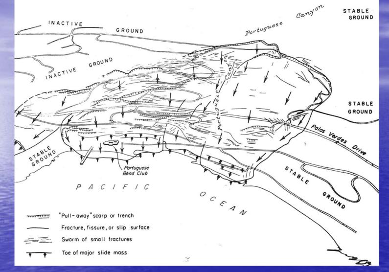
The Portuguese Bend Landslide activated in 1956, encompassing a wide area with 132 recently built homes.
