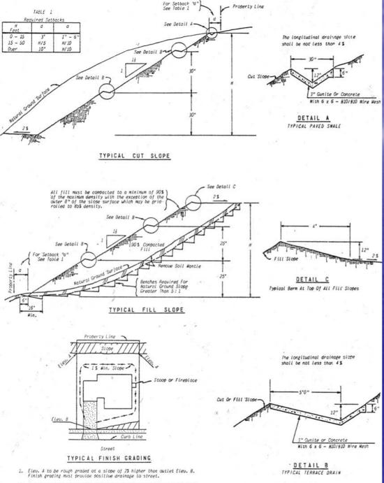
A sound suble, a catch pasin and pipe, or other similar drainage device is required when a scoop, fireplace, or portion of the building extends within 5 feet of the property line. Standards
