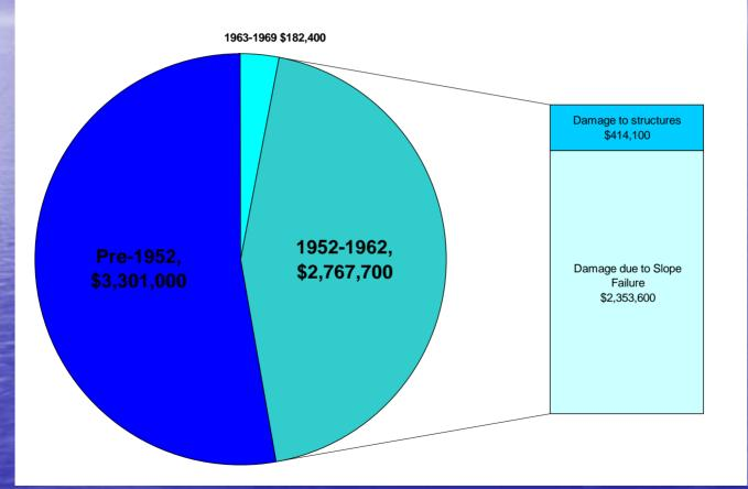
55% of damage occurred on pre-1952 structures, 40% on those built between 1952-62; prior to adoption of modern grading codes.
