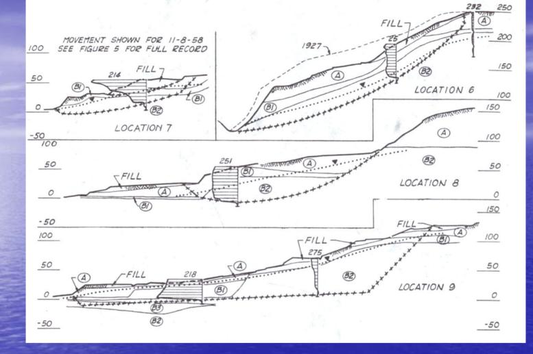
The Mueser-Rutledge study also examined mitigation options. Recompacted buttress fills became the standard mass grading technique in southern California and the Via de Las Olas slide became a city park.
