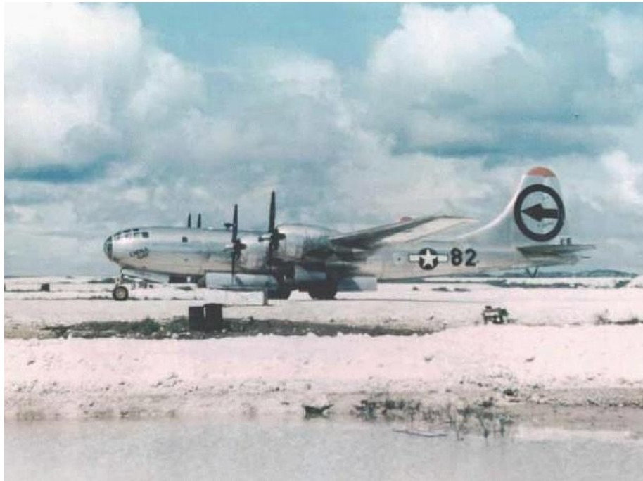
The 509 th used specially built B-29B aircraft without defensive gun turrets, which saved 7000 pounds. Only the tail guns were retained. This shows the Enola Gay wearing the arrow-in-circle tail code that was noted by Tokyo Rose in her radio broadcast a few days before the mission to Hiroshima. The 509 th tail codes were immediately changed to mimic those of regular bomb groups operating out of the Mariannas, to shield their identity.
