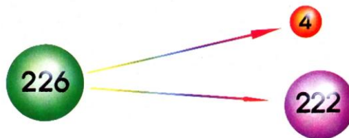
When its Alpha particle is emitted, the Radium atom falls from the atomic mass of 226 to a mass of 222 and becomes the gas Radon.
