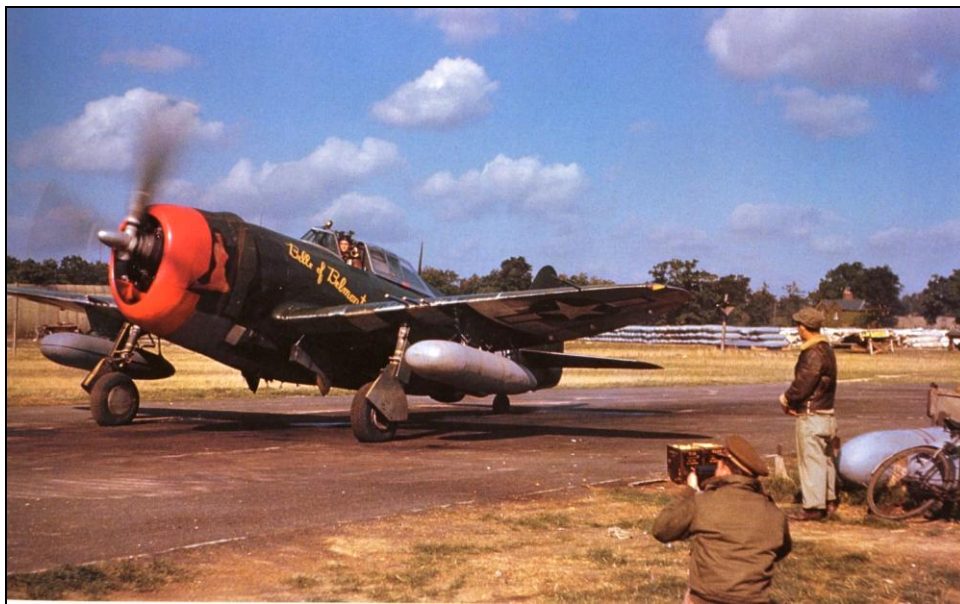
The Republic P-47D Thunderbolt was the rugged mainstay of American fighter strength in the ETO in mid-1943. It was powered by a massive 2,430 horsepower radial engine and carried eight 50-caliber machine guns in its wings. It was called a "Jug" by the Americans and "Jabo" by the Germans, who feared the terrible damage wrought by its ground strafing.
