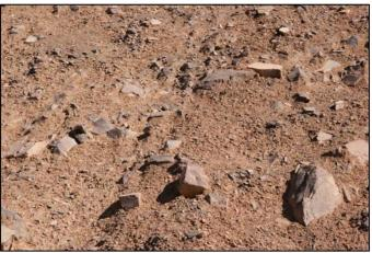
Fig. 19. - Close up of "dirty" rockfill exposed on lateral margins of the breach. The large clasts are 10-12 inches diameter.
