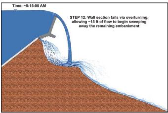
Fig. 11. – This step portrays how the parapet wall toppled in vicinity of panel 95, initiating the catastrophic failure of the reservoir by unleashing ~15 feet of flow over the remaining embankment.
