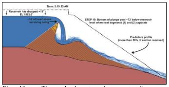
Fig. 13. – The embankment and concrete liner are progressively removed by the outflow. About one half the embankment remains at this stage.
