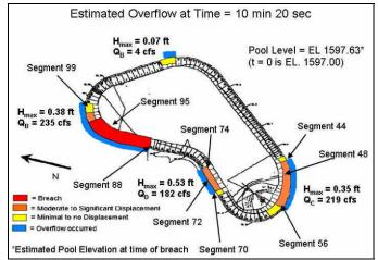
Fig. 6. – This graphic from Rizzo Associates, Inc. (2006) shows panel locations where overflow and failure occurred.
