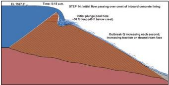
Fig. 12. – This figure illustrates ~15 feet of water overflowing
