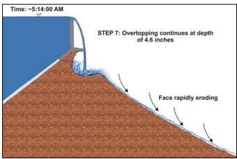
Fig 10. – This step of the reconstructed failure sequence illustrates the undermining of the parapet wall and rapid erosion of the embakment. The wall remained standing at this point due to the hydrostatic load on the inclined portion of the wall footing and 3-dimensional effects from surrounding wall panels.
