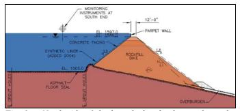
Fig. 1. – North side of the breached embankment shows the lower three quarters was end-dumped while the upper quarter was placed into two sequences of rolled filling. There does not appear to have been any significant effort made to mechanically compact the embankment because it was assumed to be a clean rockfill.
