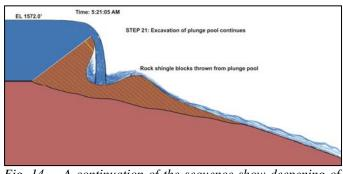
*Fig. 14. – A continuation of the sequence show deepening of the plunge pool and ejection of large shingle blocks/boulders.*
