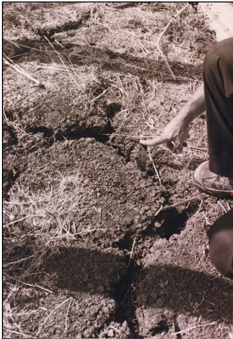
Figure 2: This crack is at least 32 inches deep. The yardstick was easily inserted to this depth; narrower, less straight cracks may extend much deeper.
