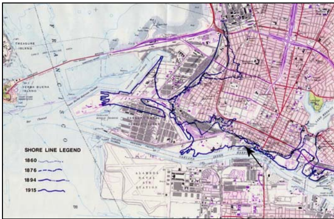
Fig. 3. Overlay of historic shorelines in Oakland, CA between 1860 and present, overprinted on USGS 1:24,000 scale DRG.
