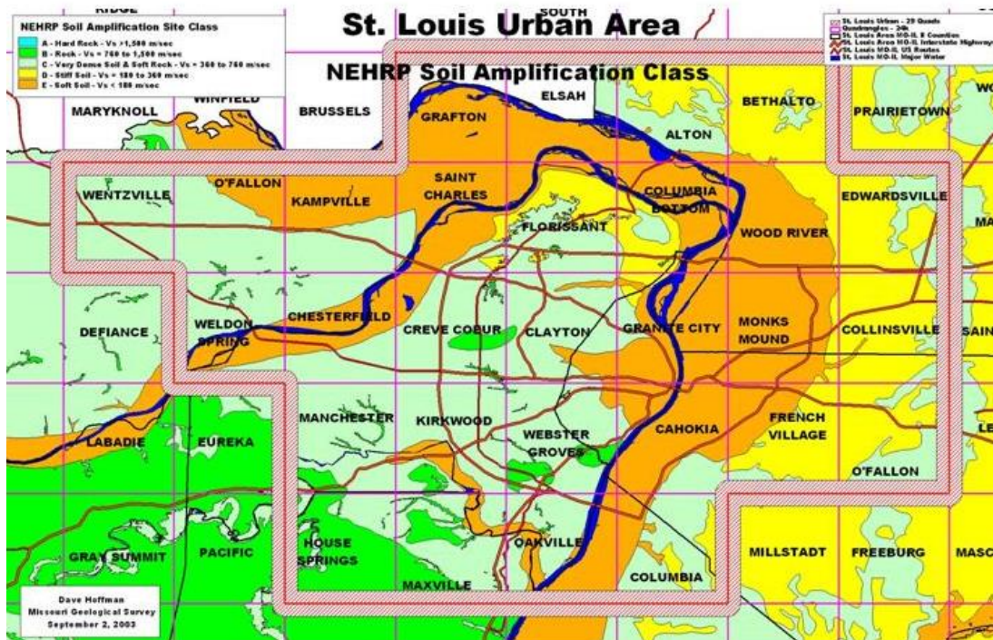
Figure 4 - NEHRP Soil Amplification Class map prepared by the Central U.S. Earthquake Consortium State Geologists. This map was prepared in 1998-99 before any shear wave velocity measurements were actually made in the area. The flood plains highlighted in orange are denoted as Soil/Site Class E, with assumed shear wave velocities of less than 180 m/sec.
